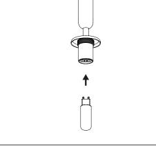
Insert a G9 light source into the socket. Make sure to press the light bulb all the way into the socket.
